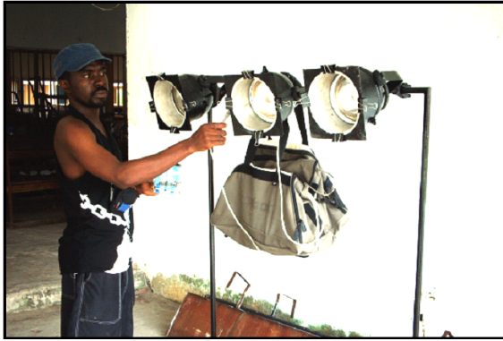
Plate 1: The researcher applying surface finishing to three studio/stage lights that he fabricated. A fabricated dimmer is housed in the bag, which enables the lights to be dimmed and brightened as required in the visual arts studio. This locally fabricated equipment, cost a small fraction of what the imported forms do. Besides, it is cheaper and easier to maintain the local technologies since foreign exchange is neither required to import parts/consumable nor to pay for expensive expatriate labour
