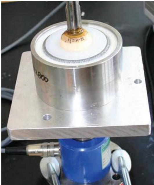
Fig.3: Torsion and axial disassembly force test setup
