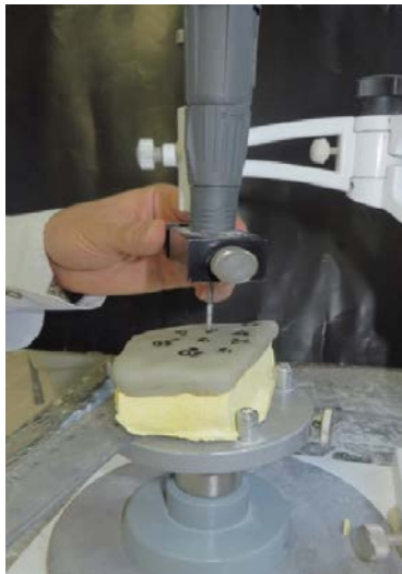
Fig. 3: Drilling stents in defined angles by a milling machine
