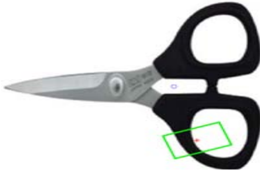
Fig. 15: Grasp point for closed scissors with a narrower gripper; X_c = 185 , Y_c = 182 , Ang = 1102 , t = 2.003006 sec
