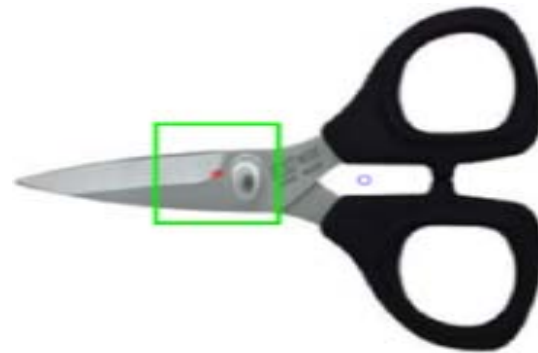
Fig. 14: Grasp point for closed scissors; X_c = 86 , Y_c = 111 , Ang = 02 , t = 1.779819 sec
