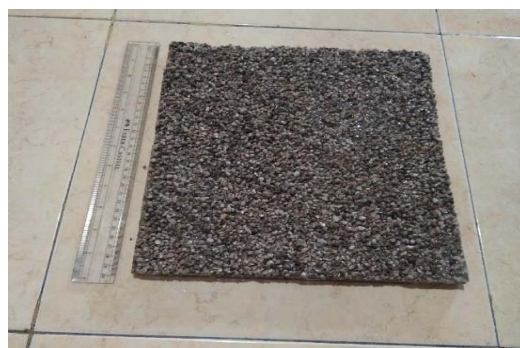
Fig. 1: Picture of pumice composite fraction sized 3 mm and weight fraction 60%
