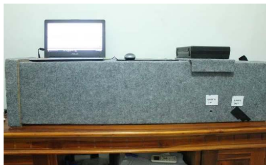
Fig. 2: Transmission loss test device
