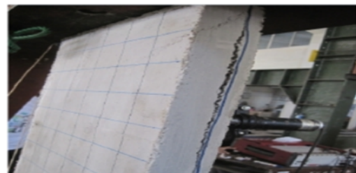
Fig. 8: Specimen of compressive test panel 3
