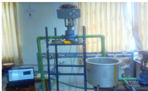
Fig. 10: Real time model of CSTR process
