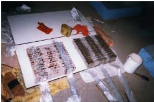
Fig. 3: Wall panels retrofitted with 2-strip and 3-strip GFRP laminations
