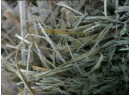
Fig. 12: Video microscope image on the crack of unboiled diss composites, magnification×25
