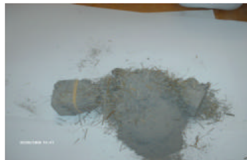
Fig. 10: Unboiled diss composite specimen after flexural test
