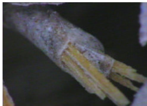
Fig. 15: Video microscope image on the crack, magnification×50
