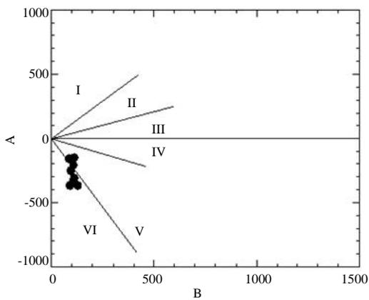
Fig. 4: B-A diagram for the granitoids after Debon and Le Fort (1983) ( $A=Al-(K+Na+2Ca)$ ,  $B = Fe+Mg+Ti$ ). I, II and III are peraluminous; IV, V and VI are metaluminous. Squares are medium grained granites, circles are porphyritic granites while the shaded triangle is potassic coarse grained granite
