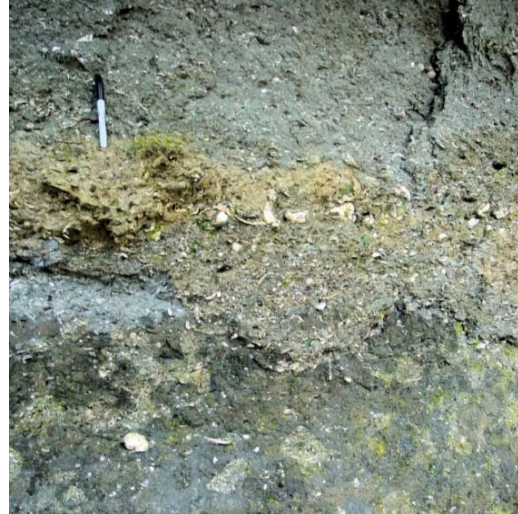
Fig. 4: PM section, the Woodstock Member of Nanjemoy Formation is unconformably underlaying the Piney Point Formation
