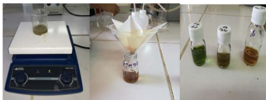
Fig. 3: Maceration with pure methanol and filtration
