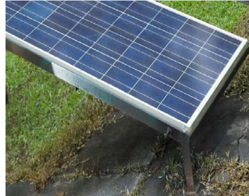
Fig. 3: Module at angle 33^\circ at North direction
