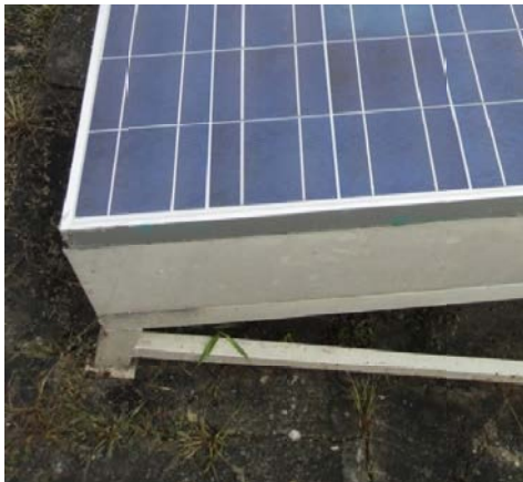
Fig. 4: Module at angle 23^\circ at north direction
