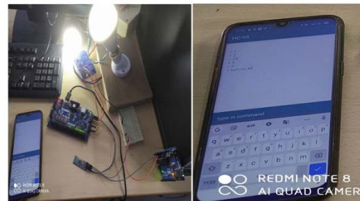
Fig. 17: Diagram for passing "turn on all" from the Arduino Bluetooth control app to the FPGA
