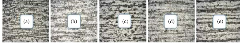
Fig. 6(a-e): Hardness of T-HRP after 30 min treatment at various R (mm): (a) 50, (b) 55, (c) 60, (d) 65 and (e) 70
