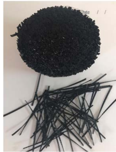
Fig. 1: Shape of macro reinforcement fibers
