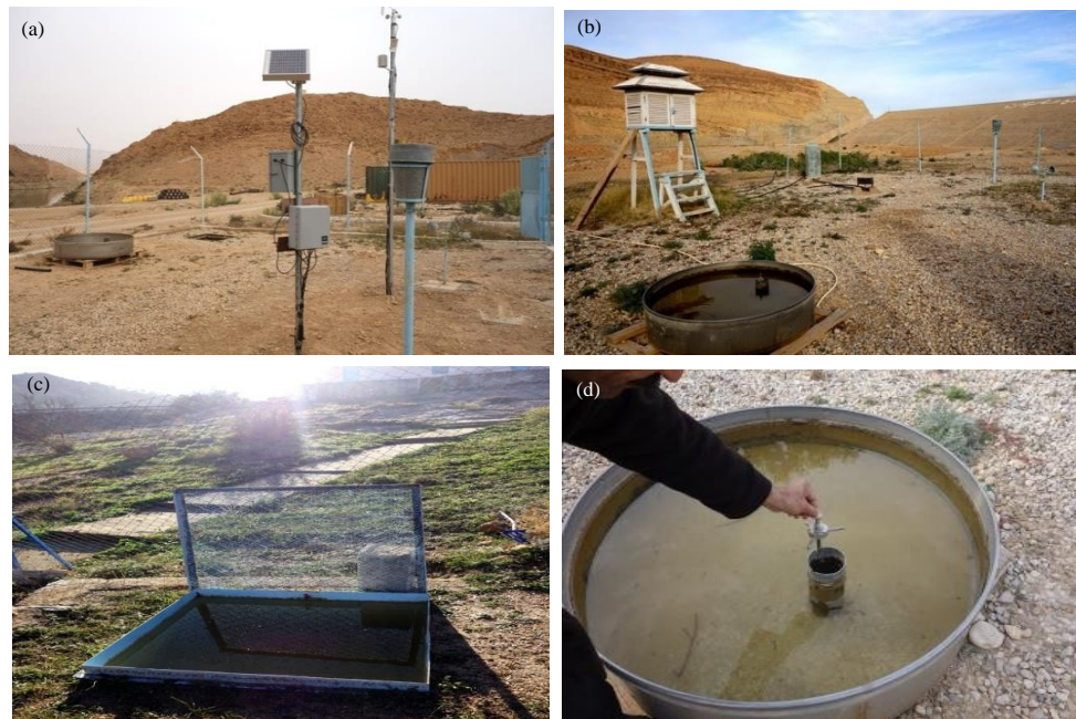
Fig. 2(a-d): Existing evaporation pans in the studied dams, (a) Weather station of Fom El-Gherza dam, (b) Weather station of Fontaine des Gazelles dam, (c) Colorado pan-Fom El-Gueiss dam and (d) Class-A-pan-Fontaine des Gazelles dam
