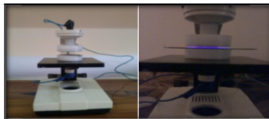
Fig. 2: Photograph of the system DBD
