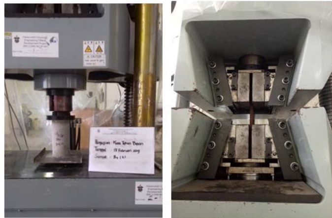
Fig. 3(a, b): (a) Cylinder test and (b) Rebar test
