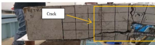
Fig. 1: The crack at the support area
