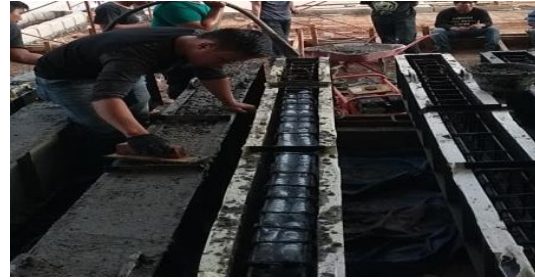
Fig. 5: Casting of specimen
