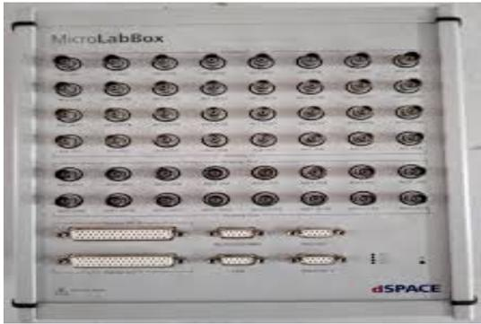
Fig. 18: dSPACE MicroLabBox (1202) controller
