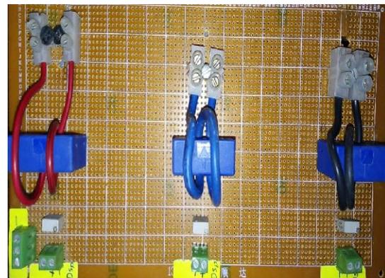
Fig. 20: Photo of the implemented current sensor board
