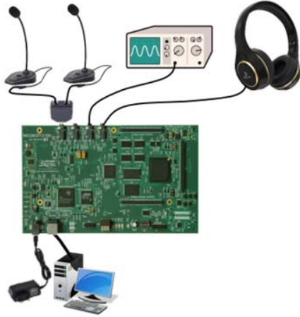
Fig. 4: Hardware setup for system separation
