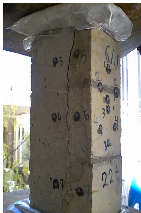
Fig. 6: Prism type b built with irregular thickness of stone units (with 100×150 mm cross section) after failure
