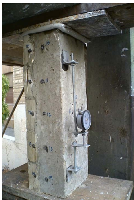
Fig. 4: Prism typed built with regular thickness of stone units (with 200×150 mm cross section) after failure
