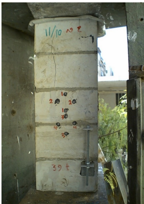
Fig. 3: Prism type d built with irregular thickness of stone units (with 200×150 mm cross section) after failure
