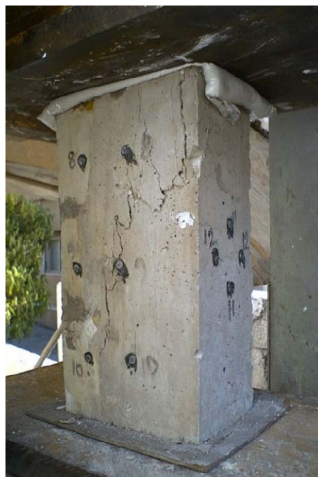
Fig. 5: Prism type b built with irregular thickness of stone units (with 100×150 mm cross section) after failure
