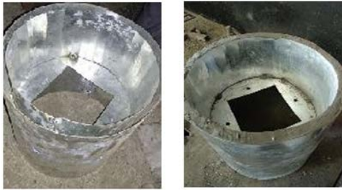
Fig. 7: Manufacturing of skirt for stove
