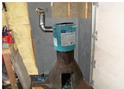
Fig. 12: Real-time proposed rocket stove
