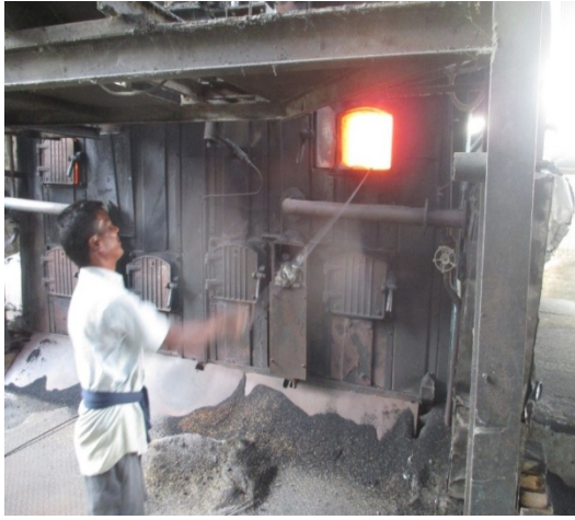
Fig. 15: Rice husk fired furnace of Asian Thai Food, Sonapur, Sunsari, Nepal
