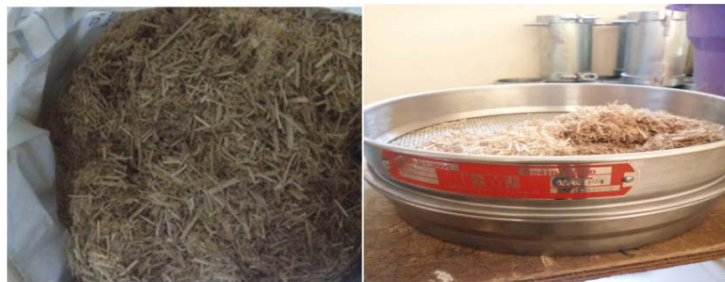
Fig. 4: Preparation of typha particle size analysis
