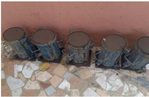
Fig. 7: Earth-only cylindrical sample
