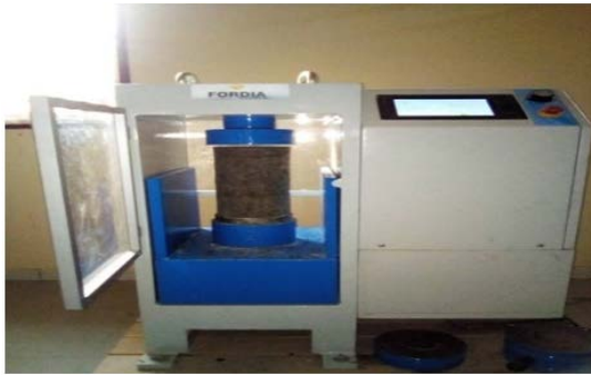
Fig. 11: FORDIA compression machine with sample
