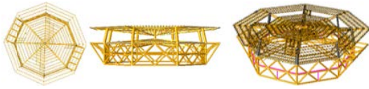
Fig. 3: Structural design modelling
