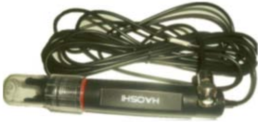
Fig. 7: pH sensor used in the automated hydroponic system
