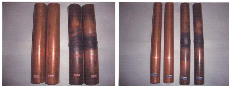
Fig. 2: Copper pipes before and after welding processes
