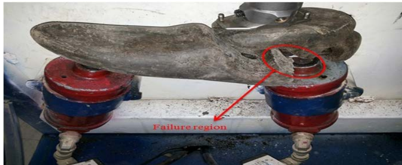
Fig. 5: Failure region in non-articulated foot (HDPE+LLDPE)
