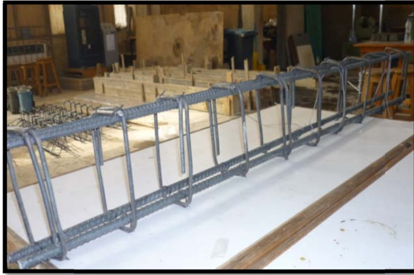
Fig. 3: Reinforcement details of beam
