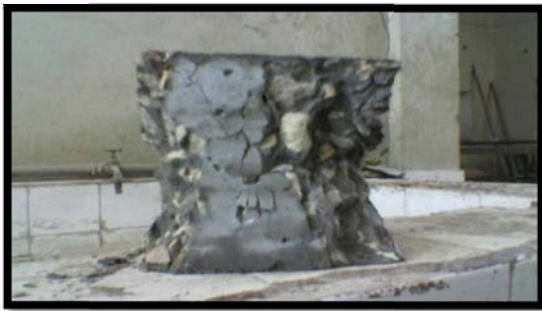
Fig. 4: Standard cube failure shape
