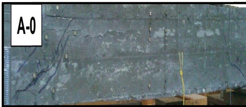
Fig. 7: Crack patterns for specimen (A-0)
