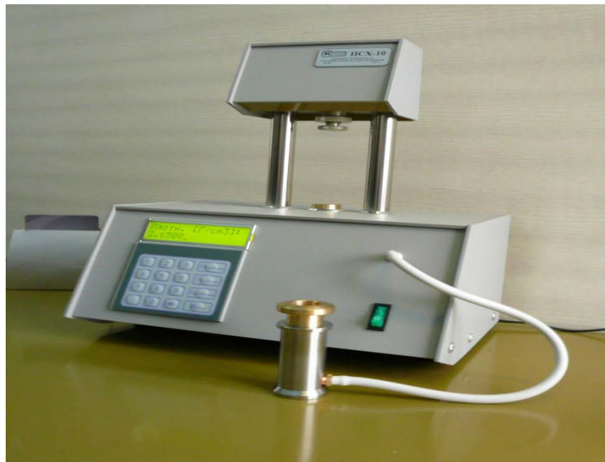
Fig. 4: Device for determining the specific surface of the PSC-10
