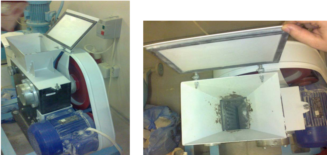
Fig. 3: A laboratory mill for grinding materials
