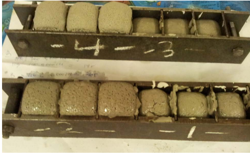
Fig. 7: Extrusion of aerated concrete samples in molds
