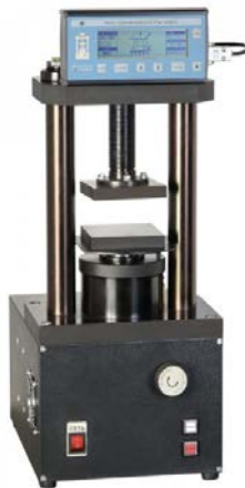
Fig. 9: Compressive strength tester
