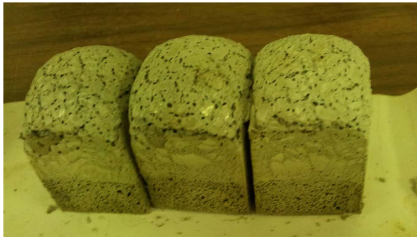
Fig. 8: Aerated concrete samples aged 1 day
