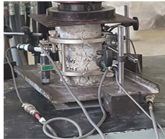
Fig. 2: Equipment for the compressive strength test
