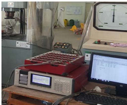
Fig. 4: A set of data loggers and computers
