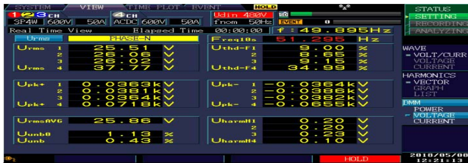
Fig. 48: Experimental results-DVR with SPWM for swell (50%) Total Harmonic Distortion (THD)
