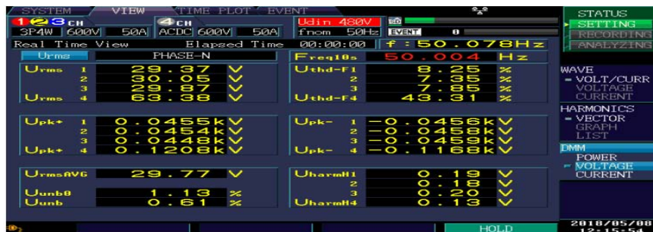
Fig. 38: Experimental results-DVR with SPWM for swell (16%) Total Harmonic Distortion (THD)
