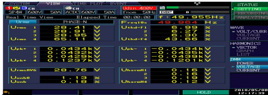
Fig. 35: Experimental results-DVR with SPWM for swell (36%) Total Harmonic Distortion (THD)
