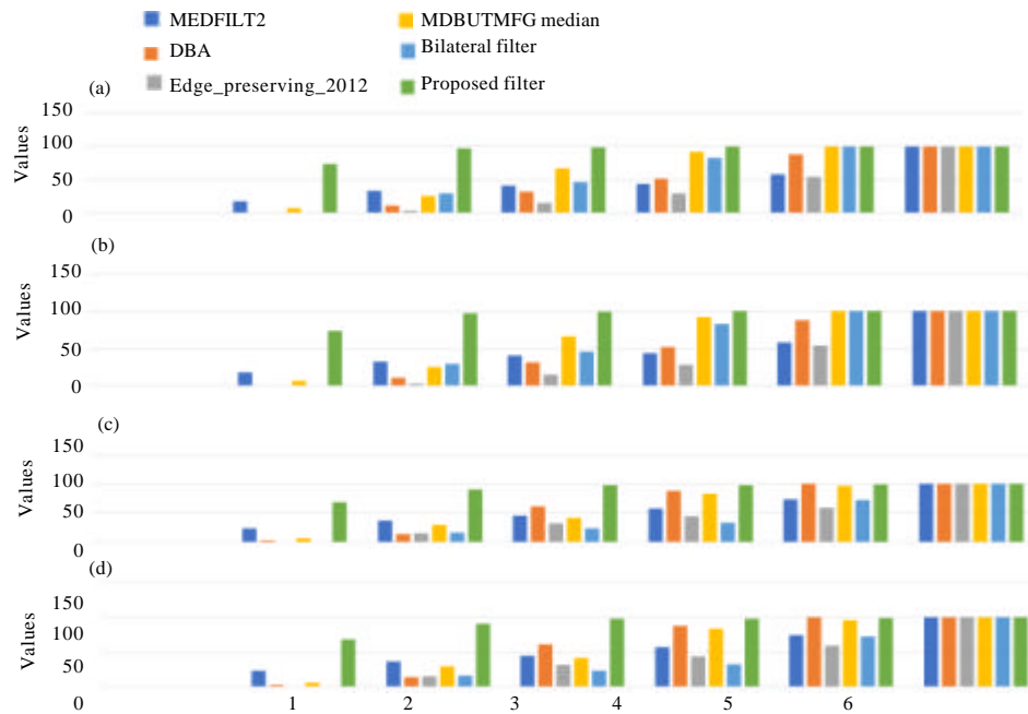
Fig. 7: Cumulative ranks for 100 test images (noise density = 0.4): a) Mean square error cumulative rank; b) PSNR cumulative rank; c) Structural similarity (SSIM) index cumulative rank and d) Multi Scale Structural Similarity Index (MS-SSIM) cumulative rank
