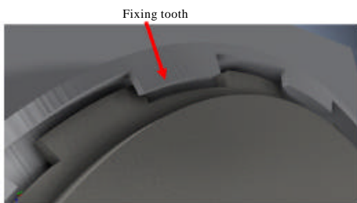
Fig. 4: Approach on the quick closing door mechanism fixing teeth
