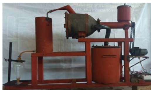
Fig. 3: The continuous-fed steam distillation essential oil extractor
