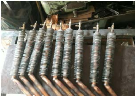
Fig. 2: Thermosyphon with 40 fins at 45° angle of inclination
