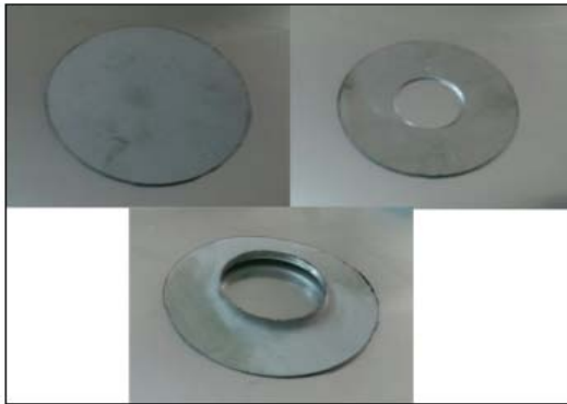
Fig. 3: Manufacture steeps of fins
