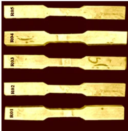
Fig. 4: Specimen for ultimate tensile strength
