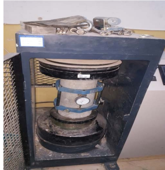
Fig. 3: Cylindrical concrete specimen under testing for stress-strain behavior
