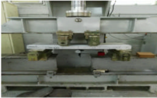
Fig. 6: Test set-up of ferro geopolymer slab
