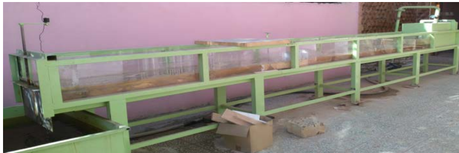
Fig. 2: The laboratory flume
