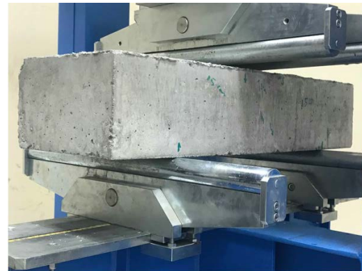
Fig. 5: Ribbed slab experimental set up
