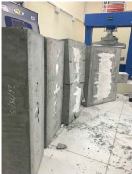
Fig. 12: Ribbed slabs of variable width after failure
