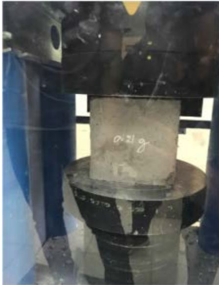
Fig. 3: Concrete cube is tested for compressive strength
