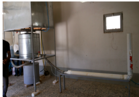
Fig. 3: General view of the hydraulic conductivity test rig
