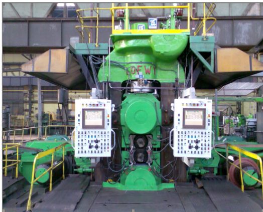
Fig. 1: Example of a reversible cold rolling mill
