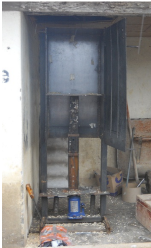
Fig. 6: Baler machine used in the project
