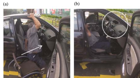
Fig. 3: Self-made upholstery to increase the seating height. The self-made modification causes a shorter driver to face difficulty reaching the pedal as well as poses visual limitations
