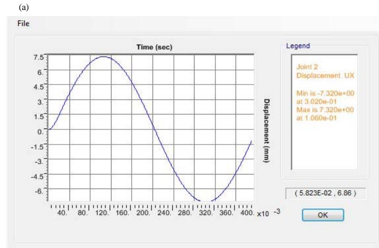
Fig. 8: a) Elasto-plastic solution at R_m = 44.76 kN using SAP (Ver. 18) and b) Responses of elasto-plastic structure ( R_m = 44.76 kN) and purely elastic structure ( R_m = 44.76 kN)
