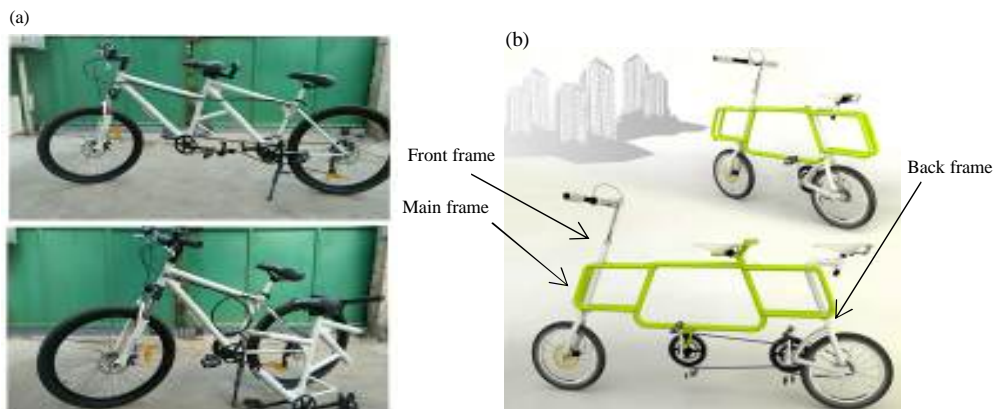
Fig. 1: a) Tandem bike, the bike could be used as the tandem bike or the single bike based on the need and b) The sliding tandem bike again it could be transformed to the tandem or single bike with only reposition of front and back frame on the main frame (Iskandriawan and Jatmiko, 2014; Iskandriawan et al. , 2017)
