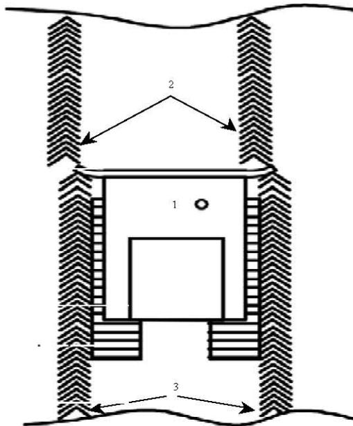
Fig. 4: Scheme of the bulldozer movement that ensures minimal losses of load during its movement: 1: Bulldozer; 2: Rolls remaining from the previous passage and 3: Newly formed rolls
