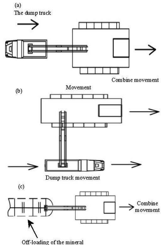
Fig. 1: Scheme of work of a milling combine; a, b) With the loading of the mineral into the dump truck and c) Off-loading of the mineral into the dump
