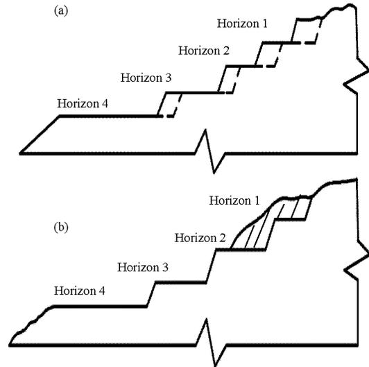
Fig. 3: Scheme of blasting operations: a) Before blasting and b) After blasting
