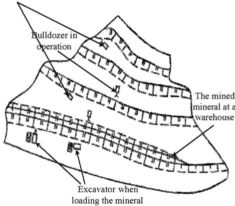
Fig. 2: Scheme of exploitation using a bulldozer and an excavator
